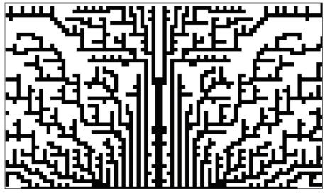
Figure 2: Heatsink profile after one 'year' of growth.
