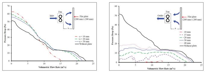
Note: a = separation distance between fan and flat plate obstruction.
