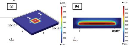
Figure 3: . FE temperature profile after 0.5 s for (a) FCBGA package and (b) the A-A cross section (dimensions in m, temperature in K).
