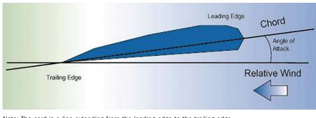
Note: The cord is a line extending from the leading edge to the trailing edge. Angle of attack is the angle formed between the relative wind and chord.
