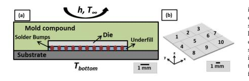
Figure 2: Simplified schematic of (a) FCBGA package used in this study for package level modeling and (b) the enclosed die with function blocks for chip level modeling.
