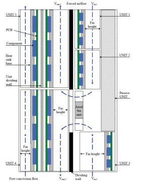
Figure 1: System geometry and internal airflow patterns.
