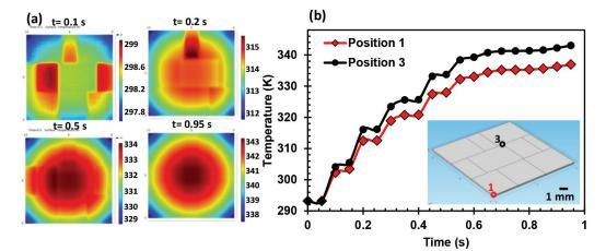
Figure 5: (a) Spatial distribution of temperature profile at chip level on top of the transistor layer after 0, 0.1, 0.5, and 0.95 s, (b) temporal distribution of temperature at two locations on the chip.
