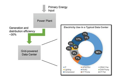
Figure 1: Energy Flow for a Conventional Grid-Powered Data Center.
