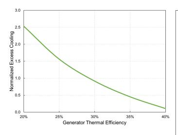
Figure 4: Data Center Excess Cooling Available for the Example Cogeneration System Data Center.
