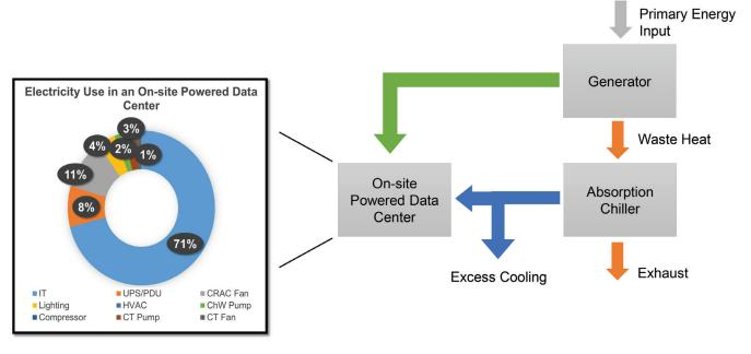
Figure 2: Energy Flow for an On-Site Powered Cogeneration Data Center.
