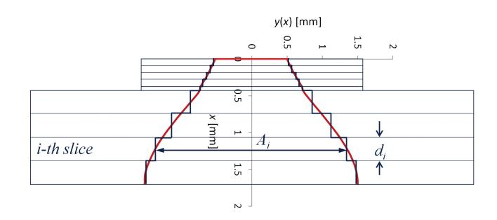
Figure 4: Discretization of the effective heat spreading cone.
