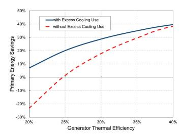
Figure 3: Primary Energy Savings for the Example Cogeneration-based Data Center.
