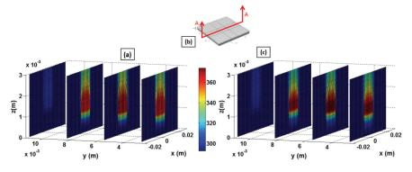
**Figure 4:** Temperature profile inside the package at 1 s extracted from the POD model (a) and FE simulation (c). The domain is sliced vertically along XZ plane. The right-most slice is the A-A cross section (b) (adapted from [11]).
