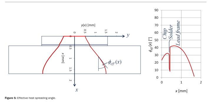
good approximation for a whole sub-class of cases (*e.g.* all power semiconductors with solder die attach). Based on these rules and *Equation* (5) we can implement more accurate spreadsheet calculators for the thermal resistance of this sub-class of devices.
