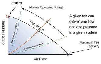
Figure 3: Fan/system interaction.
