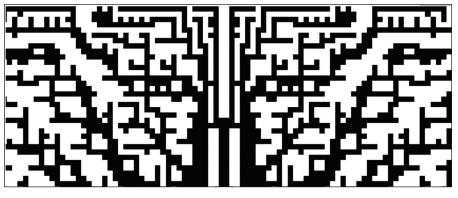
Figure 3: Forced convection heatsink profile after three 'years' of growth.
