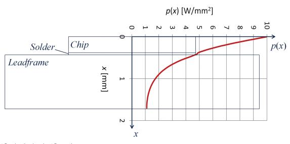
Figure 2: Heat flux density along heat flow path.
