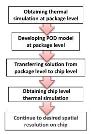
Figure 1: Flowchart of the hybrid scheme
